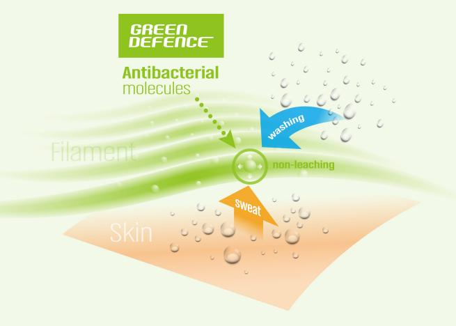
Under the polymerization process at a temperature of more than 480°F, cinnamon and almond extract are blended into polyester or nylon. Therefore, the particles will not leach out during washing and at use. GREEN DEFENCE is all natural, non-leaching and can provide consumers overall protection.
